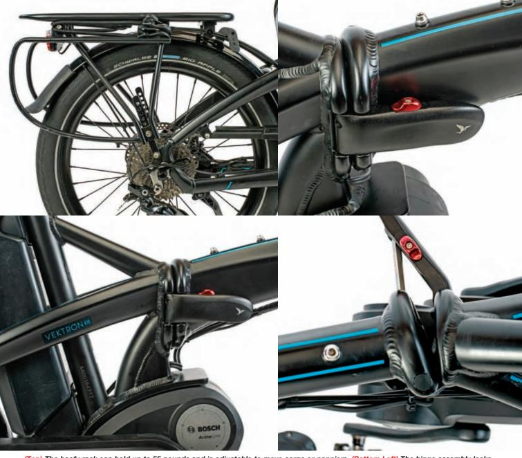
(Top) The beefy rack can hold up to 55 pounds and is adjustable to move cargo or panniers. (Bottom Left) The hinge assembly locks solidly and folds flat when open or closed. (Bottom right) This bike is so solidly built, you'll forget it's a folding bike. It has structural braces everywhere.
