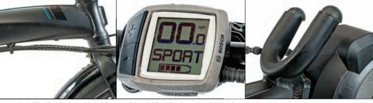
(Left) All cabling is external, which is unusual for a folding bike these days. (Middle) A Bosch Purion display puts everything you need at your fingertips, but you may have to reposition it so the sharp edge doesn't cut into your hand. (Right) This little horseshoeshaped piece protects the motor and allows the bike to stand when folded up.
